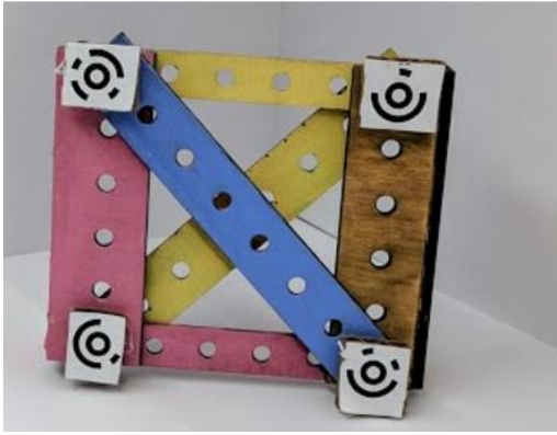
Figure 4 Sample Construction with Topcodes at Joints
